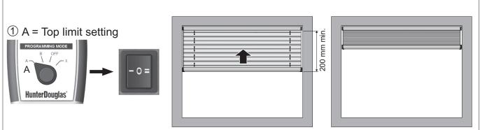
Blind must be down at least 200 mm before setting top limit. Press I or II and hold until the blind stops by itself.
