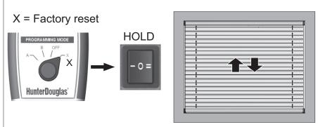
Press and hold I or II until the blind moves (for 5 seconds)
